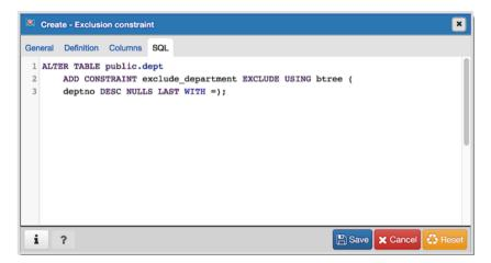
The example shown demonstrates creating an exclusion constraint named *exclude\_department* that restricts additions to the dept table to those additions that are not equal to the value of the *deptno* column. The constraint uses a btree index.
