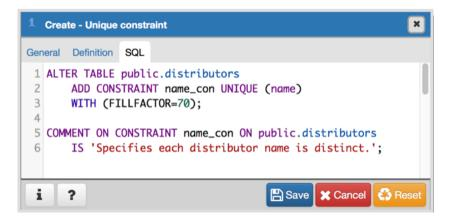
The example shown demonstrates creating a unique constraint named *name\_con* on the *name* column of the *distributors* table.
