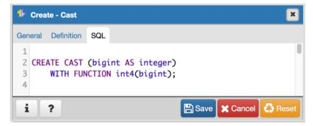
The cast uses a function named int4(bigint) to convert a biginteger data type to an integer.
