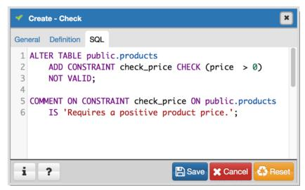
The example shown demonstrates creating a check constraint named *check\_price* on the *price* column of the *products* table. The constraint confirms that any values added to the column are greater than 0.
