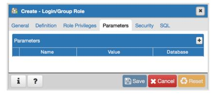
Use the fields on the *Parameters* tab to set session defaults for a selected configuration parameter when the role is connected to a specified database. This tab invokes the ALTER ROLE... SET configuration\_parameter syntax. Click the *Add* icon (+) to create a parameter.
